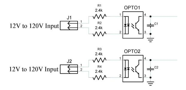
The image above shows inputs 1 and 2. The input impedance for each input is 4800 Ohms.
