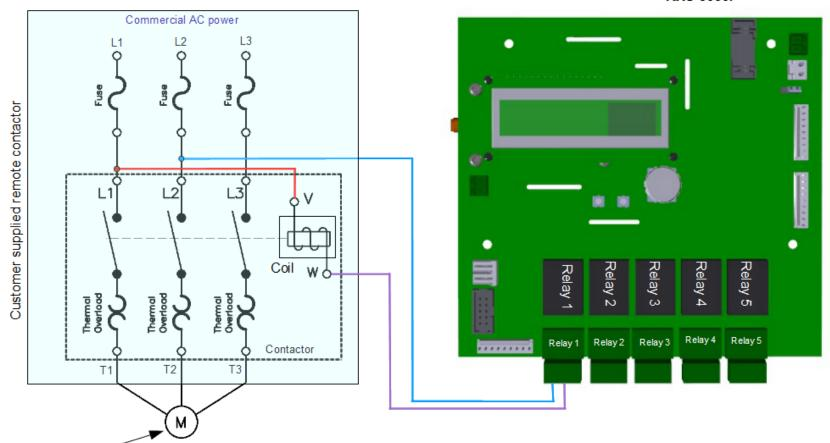
Customer's motor, light, resistive or inductive load
