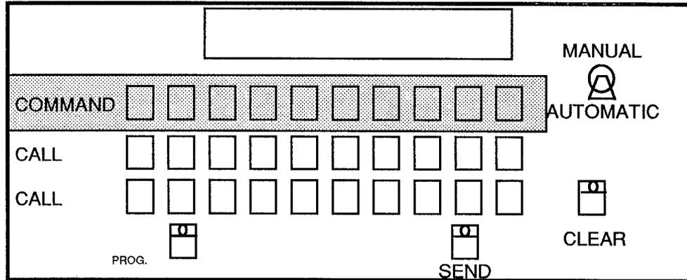
After you press any key in the COMMAND row of keys, the display screen will change from the READY \_ indication. It will now display CALL COMMAND ?. The KEYS is for the second line of the display to show which of the CALL keys are going to be sent. The COMMAND ? will show which COMMAND key you pressed to be sent. If you pressed COMMAND key 2 the display will show COMMAND 2.
