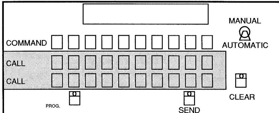
Example, if CALL key "A" called unit 1, CALL key "B" called unit 2, and so forth. To activate unit 2 you would press the CALL key labeled "B". The letter "B" would show on the second line of the display indicating that that CALL code would be sent when you press the SEND key.
