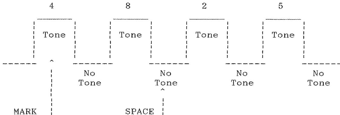
Each tone MUST have a duration long enough to allow the receiver time enough to decode it, plus there must be enough Space between the tones so that the decoder can understand that one code is ending and another is beginning.
