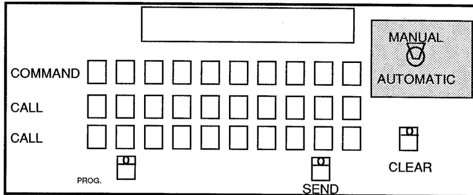
Whenever you want the Encoder to Stop what it is doing and Clear the MANUAL Mode screen, or to just Clear the screen, press the key labeled CLEAR.
