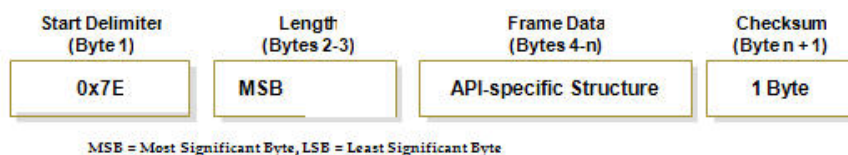
Figure 5-01. UART Data Frame Structure
