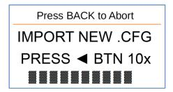
Used to read the CFG file from the SD card. The CFG file holds the configuration of the MP3 node. When cloning nodes or changing configuration of multiple nodes, reading the CFG file is the easiest method to make changes.
